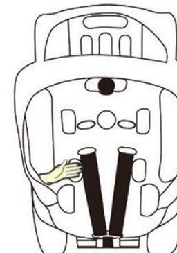
Step 1: as shown, retreat the shoulder belt from the connecting steel of shoulder belt on the back of child safety seat, retreat two shoulder belts from the splayed hook piece, pull shoulder belts from the seat in front, then take the upper part of shoulder belt down.
