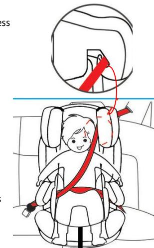
Step 1: put the child safety car seat in a car with three-point seat belt and make sure the backrest close to the car seat.
