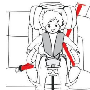
Step 7: as shown in the figure, put the child in the safety seat (the children older than two years should not use mattress), lock the buckle and tighten the front drawstring.. Tighten the lap-belt under the precondition of ensuring the comfort of child.
