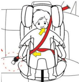
Step 3: as shown in the figure, plug shoulder harness and belt into the safety slot of car. The sound of click is heard. Pull the lap-belt up and check whether it is locked. Ensure shoulder belt and waist belt pass by under the handrail. Check whether the safety belt of car is bent or twisted. Tighten the seat belt along the direction of arrow.
