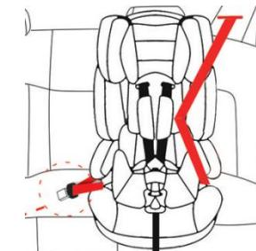
5. As shown in the figure, lock the lap-belt in the front of car under the handrail at the same side, then plug it into the groove of lap-belt leaving a sound of click. Check whether it is locked properly by pulling the safety belt up.
