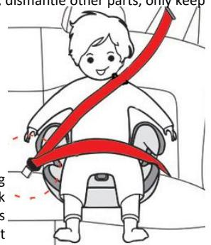
Step 2: lock the seat belt in the slot of seat belt leaving the sound of click. Pull the seat belt up and check whether it is locked. Ensure that the shoulder harness of seat belt passes by the top of handrail and the waist belt passes by the handrails on the both sides of seat.
